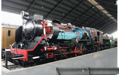
Of particular interest was a stripped down loco which allows visitors to view all the working parts. This is a permanent display which allows anyone with interest in engineering to view the complex innards of the engine.
