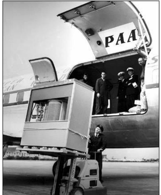
Weighing in at 1 ton, in 1956 the 305 RAMAC was the first computer in the world with a hard disc drive. There were 50 discs 600 mm in diameter. With a massive 5Mb of storage it would not quite cut it today: we can hang 1000 times that on a key ring.
