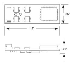
**NOTE:** Model DSD-100LC is designed to work at N and HO track settings only. Not for use with track voltages above 16 volts.
