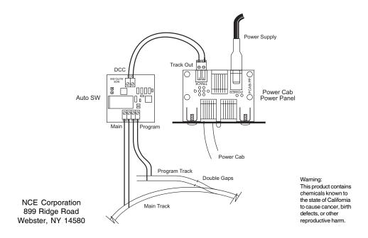
When the Power Cab is changed to "USE PROGRAM TRK", the entire main line becomes the program track. You could end up with all of your locomotives having the same address.
